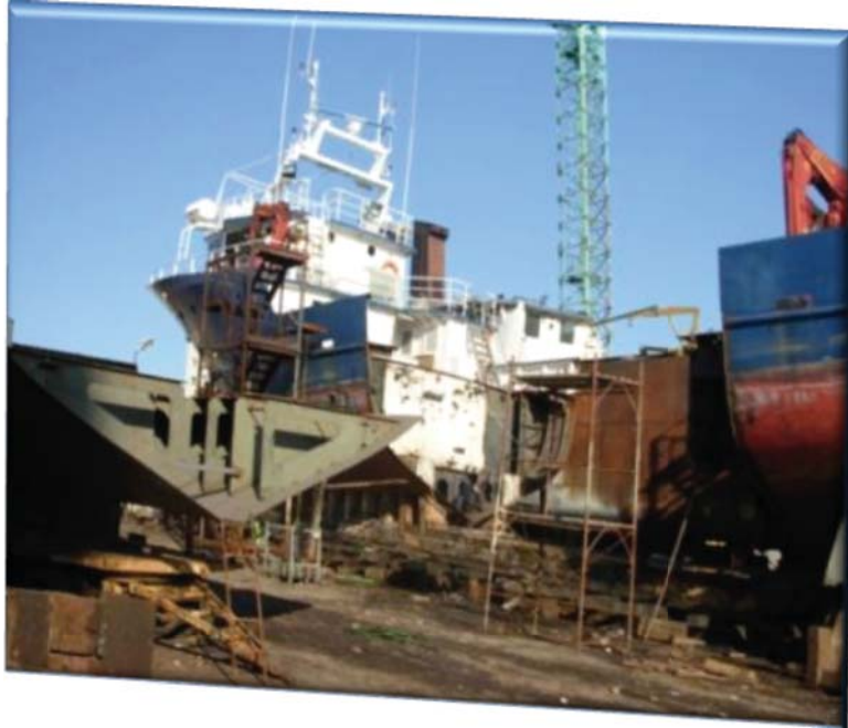
Figure 009: 10m LOA jumborization of Italian flagged BFT PS vessel Eureka (Società Euromar di Ganesio Pietro) by 10m. 2004. Picture: Courtesy by Cantieri Navali Megaride©©, Naples, Italy.
